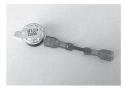
Example: Attic temperature rises to 80° and fan turns on. Once it cools to 65° the fan will shut off. If evening comes and temp does not fall below 65° to reset the switch, then the unit will start the next morning at sunrise and continue to cool the attic. However, if the attic temp falls below 65° at night, then the switch will shut off and will not turn the unit on again until attic temp reaches 80°.
