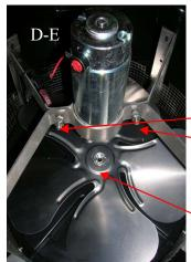
Loosen these 2 bolts to slide motor.
